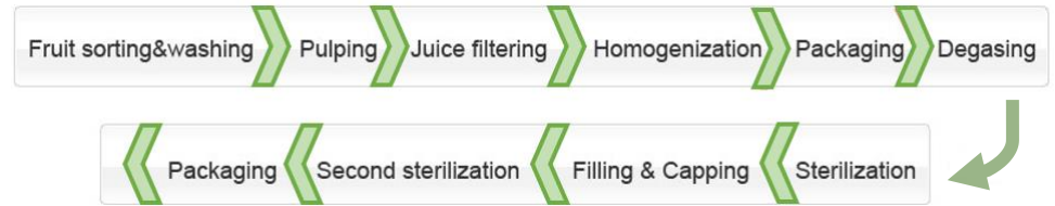
General schematic flowchart of fruit juice processing.
